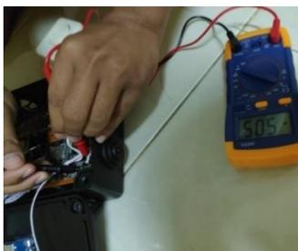
Gambar 3 Pengukuran DC Power Supply
