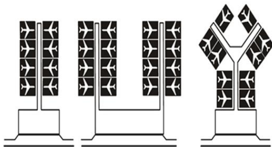
Gambar 8 Pier Concept (Doc 9157-AN/901 Aerodrome Design Manual Part 2 Taxiway, Apron and Holding Bay, Fourth Edition, 2005, chapter 3.3.3)
