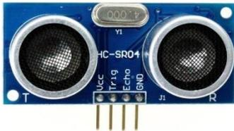
Gambar 5 Sensor Ultrasonik
