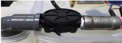
Gambar 18 Sensor Flowmeter
