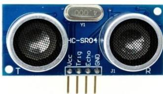
Gambar 4 Sensor Ultrasonik HC – SR04
