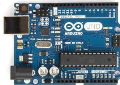
Gambar 2 Board Arduino Uno R3
