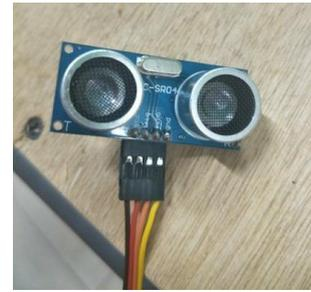
Gambar 17 Sensor Ultrasonik
