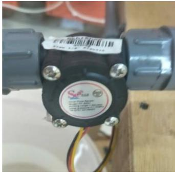
Gambar 20 Sensor flow meter
