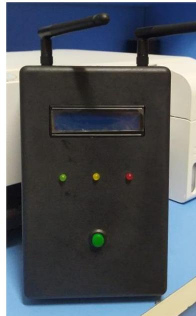
**Gambar 3** Tampilan Prototipe *Airbone Marker Beacon*
