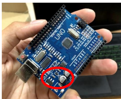
Gambar 8 Port Input Power Arduino Uno Dilepas
