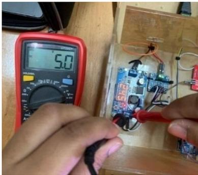
Gambar 4. Pengujian *Port Output Power Supply*
