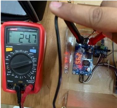
Gambar 3. Pengujian *Port Input Power Supply*
