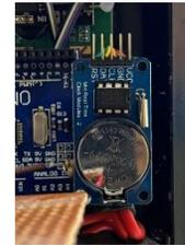
Gambar 2.5 Real Time Clock (RTC)
