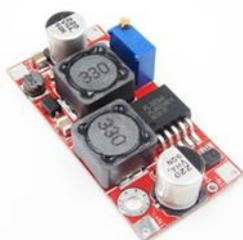
**Gambar 5** Buck Boost Converter
