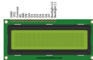
Gambar 2. 5 LCD (Liquid Crystal Display)
