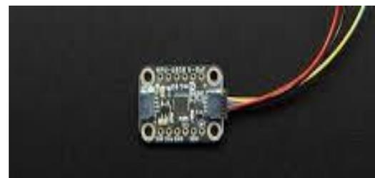
Gambar 8 Sensor Gyro MPU6050
