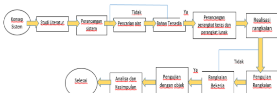
Gambar 1 Bagan Metode Perancangan Sistem Monitoring Voltase Battery
