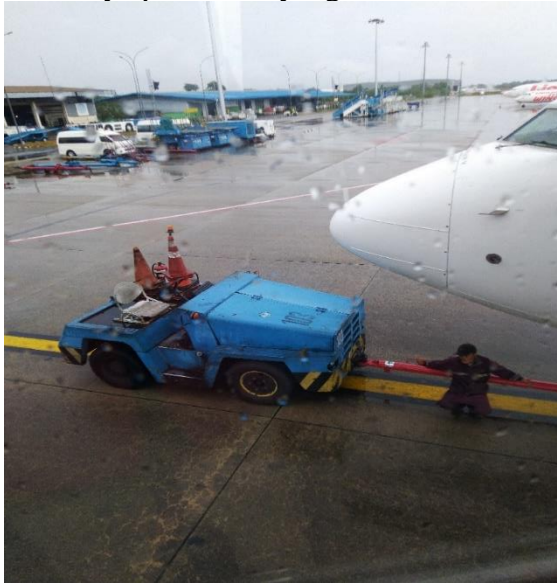
Gambar 3 Aircraft Towing Tractor yang Berkarat di Parking Stand AE 6
