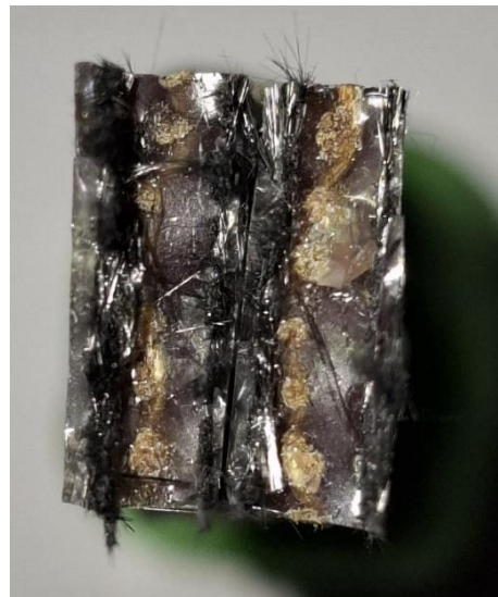
Figure 9. Specimen C Fracture
