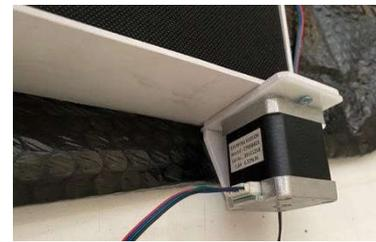
**Figure 12** Nema 17 BLDC Stepper Motor
