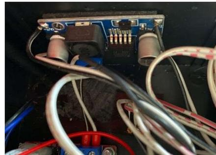
**Figure 13** Buck Converter LM2596
