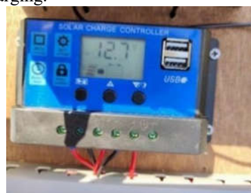
Figure 3.2 SCC (Solar Charge Controller) Testing
