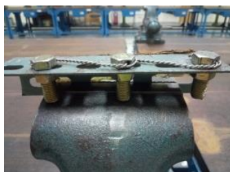
Gambar 3. Kondisi Awal Safety Wire
