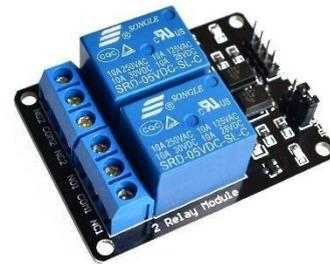
**Gambar 3. Relay 2 channel**
